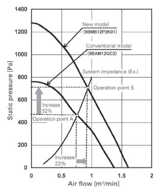
Fig. 5: Comparison of air flow and static pressure
