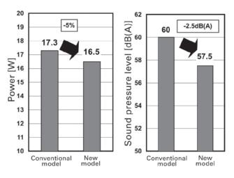
Fig. 7: Power consumption and sound pressure level comparison at operation point A
