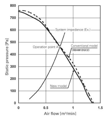
Fig. 6: Comparison of air flow and static pressure (Conventional and new model at same operation point)
