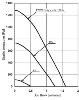
Fig. 3: 9BMB12P2K01 Air flow vs. static pressure
