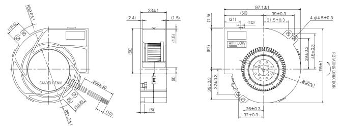
Fig. 2: "San Ace B97" BMB type dimensions (unit: mm)
