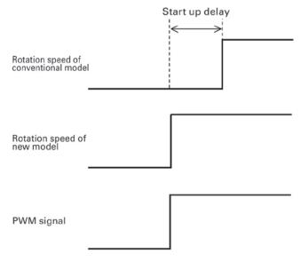
Fig. 8: Scheme of PWM strating signal
