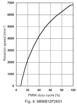
PWM duty cycle and speed characteristics
